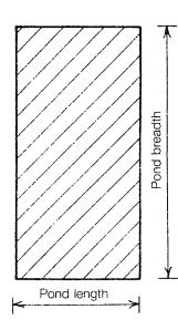
The inlet to a series of ponds should be constructed in concrete to prevent bank erosion, and should be designed so that sewage enters below top water level. In order to ensure that the pond contents are well mixed by winds the ratio of breadth to length should be in the range 1:2 or 1:3.
