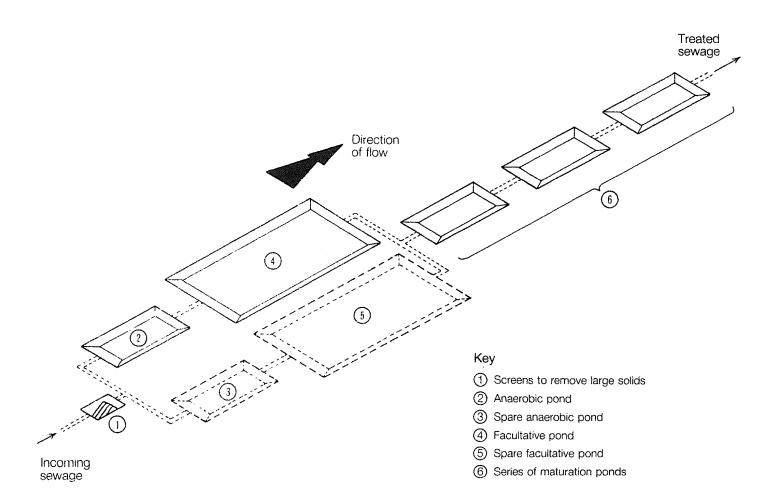
So that any pond may be isolated for maintenance work or to allow sludge to be removed, at least one extra pond of each type should be provided.
