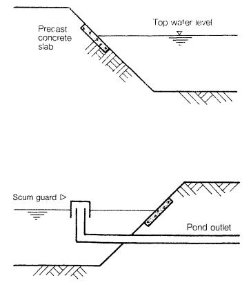
Pre-cast concrete slabs should be laid at top water level around each pond to discourage growth of weeds and to prevent bank erosion caused by wave action.
